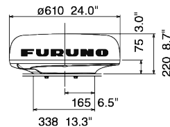
24" Radome Radar Sensor DRS4DNXT 7.3kg 16.1 lb
